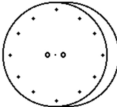
Make 2 washers 2" in diameter with a 1"1/4 hole. Use 1/8" masonite.
