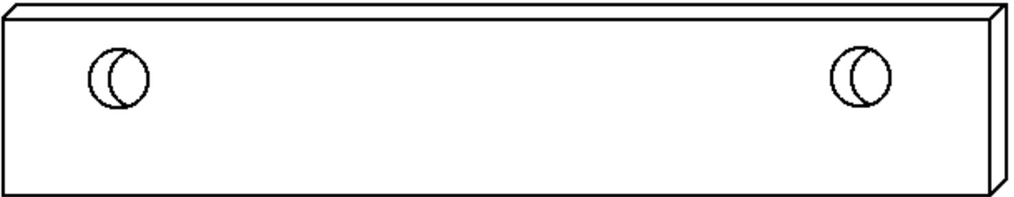
In each side rail drill 2 holes that are 1"1/4 in diameter. You may have to enlarge these slightly so that the rollers can turn freely in them. Center the holes 2"1/2 from each end and down 1"1/4 from the top edge.
